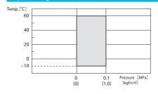
Use after confirmation that the maximum operation pressure and maximum service temperature are within the operation range.
