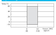
Use after confirmation that the maximum operation pressure and maximum service temperature are within the operation range.
